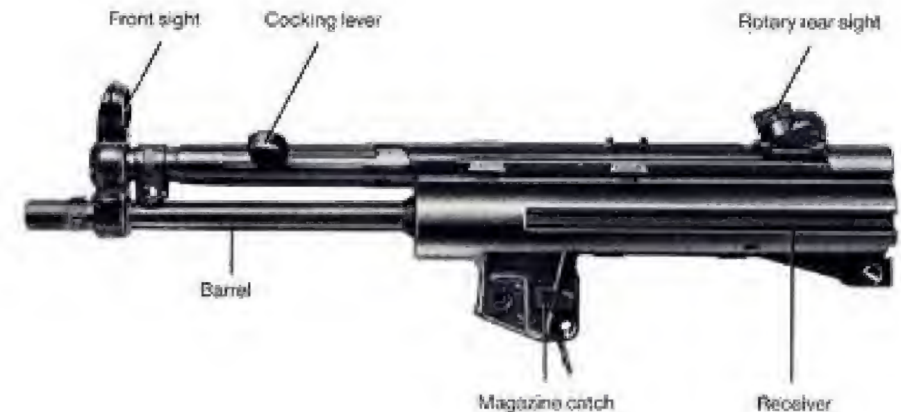
Fig. 4 Receiver with barrel, cocking mechanism and sights
